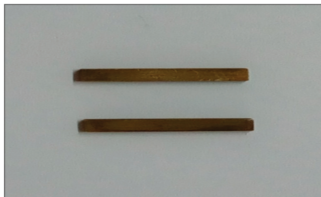
Figure 1: Brass die 2 mm × 2 mm × 10 mm
